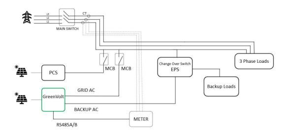
Practice 2: New Installation of two GreenVolt in a 3PH-system
